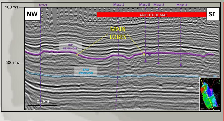
Strike PSTM seismic section showing two major lobed shapes interpreted as turbidite lobes. Each of these features shows seismic evidence of differential compaction and have their feeder systems to the east-northeast.
