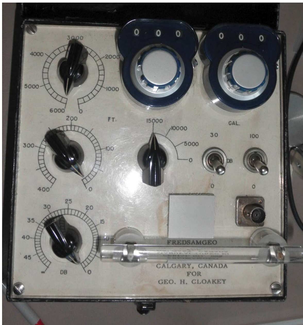
Figure 5. The classical “black box” doodlebug, from the collection of long-time Calgary landman Ned Gilbert. This radionics-type instrument was used to search for oil in Alberta in the 1950s. The box is filled with neatly wired electrical components of that era but has no way to connect to an electrical power source (Photo by the author).
