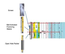
**Ball-Activated Fracturing Completion System (BAFCS)**
