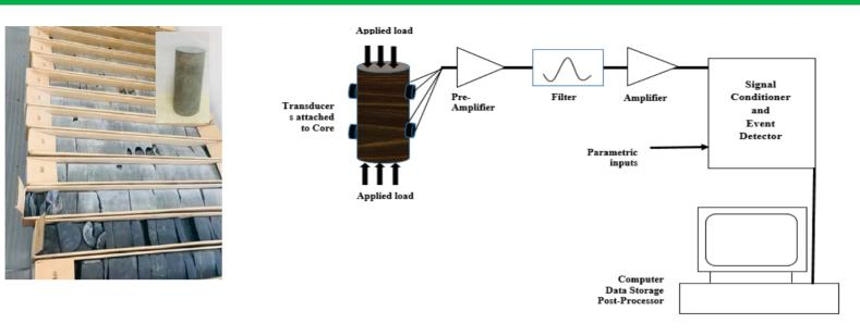
Experimental set up of acoustic emission monitoring, modified from Zhou et al (2018). This equipment will be used to measure V and S waves velocities to know how cracks are propagated on core plugs before and after CO<sub>2</sub> exposure, and to study how CO<sub>2</sub> sequestration will alter the porosity, permeability and hence the velocity of the rock.
