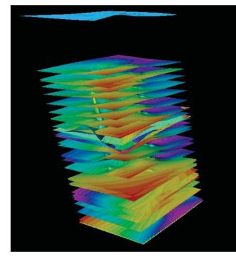
Build and geological model of the field with all the formation properties. Run a simulation of CO<sub>2</sub> sequestration in the geological model to determine its injectivity, capacity, caprock integrity and potential for fault reactivation in the basin.
