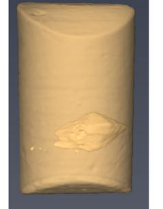
XCT scans of the core (5690.25'), a 3D image of the core and its inclusion was constructed for two different orientations. Aviso software was used to render a 3D image from XCT scans of sample 5690.25', including a partly infilled vug.
