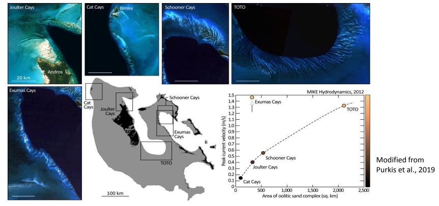
Predictive relationship from modeling in that doubling the peak current velocity increases the area of the sand body by a factor of three
