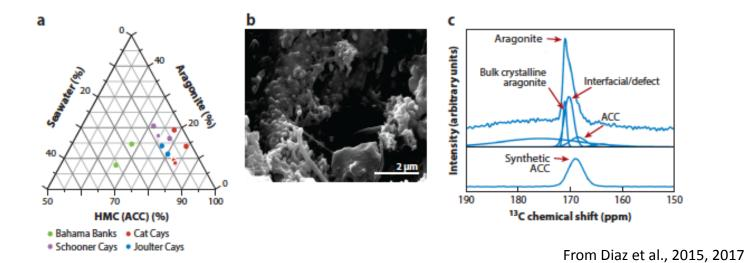
Leached geochemical signature, SEM, and nuclear NMR spectrum of ooids provides evidence for ACC in ooids and association with organic matter.
