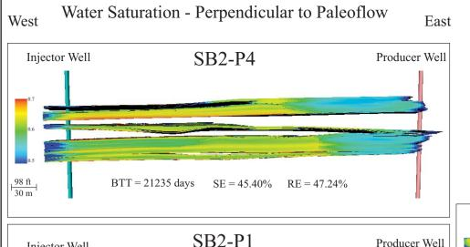
Reservoir models are placed at Burro Canyon Formation subsurface conditions and simulated using a waterflood from an injector to producer well. Simulations were analyzed for breakthrough time (BTT), sweep efficiency (SE) and recovery efficiency (RE)
