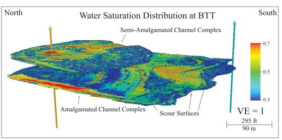
Three-dimensional water saturation model showing distribution of waterflood thorughout the reservoir. Amalgamated channel complex is the most prolific architectural element, providing higher net-to-gross ratios and a larger sandstone body connectivity.
