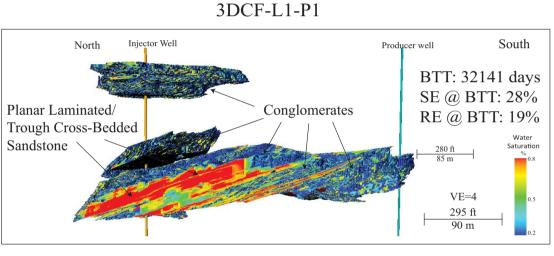
Side view comparison of two simulated 3-D models. Planar laminated and trough cross-bedded sandstone show the highest water saturations in both models, conglomerates shwos singificant decrease in water saturation in cemented model. Extent of the waterflood through the reservoir is lessened in the semi-amalgamated complexes. Sweep efficiency increases by 28%.
