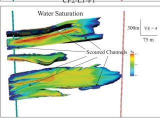
Comparing three levels of internal heterogeneity, SB2-P1 which has no internal heterogeneity, SB2-P4 which uses a "tank" petrophysical distribution, and CF2-L1-P1 the most heterogeneous model, waterflood at breakthrough time is shown. Internal heterogeneity decreases sweep efficiency and recover efficiency while shortening breakthrough time by creating fluid-flow pathways
