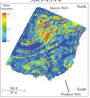
Top view of the two 3-D waterflood simulations performed. Top shows petrophysical distributions from the Mitchell Energy Federal 8-1 well. Bottom shows cemented conglomeratic facies. water saturation of the reservoir significantly decreases when cement is applied. scour surfaces observed contain little to no water saturaiton, reducing fluid flow pathways.
