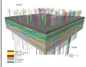
Three-dimensional models were created using 151 pseudo wells. 127 of these pseudo wells are tied directly to outcrop using a 30-foot sspacing along exposed Burro Canyon Formation, remaining 24 wells are used to constrain interior of canyon without exposures present.
