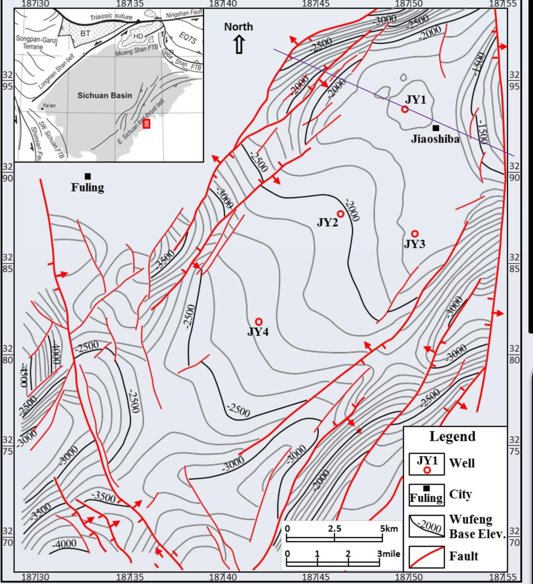
Fuling Gas Field is a anticline with many boundary faults. Our well data is from 9 wells (1 vertical well and 8 horizontal wells) in the northern Fuling Gas Field, including conventional log data, well location, and well trajectory. In addition, one well has ECS log also.
