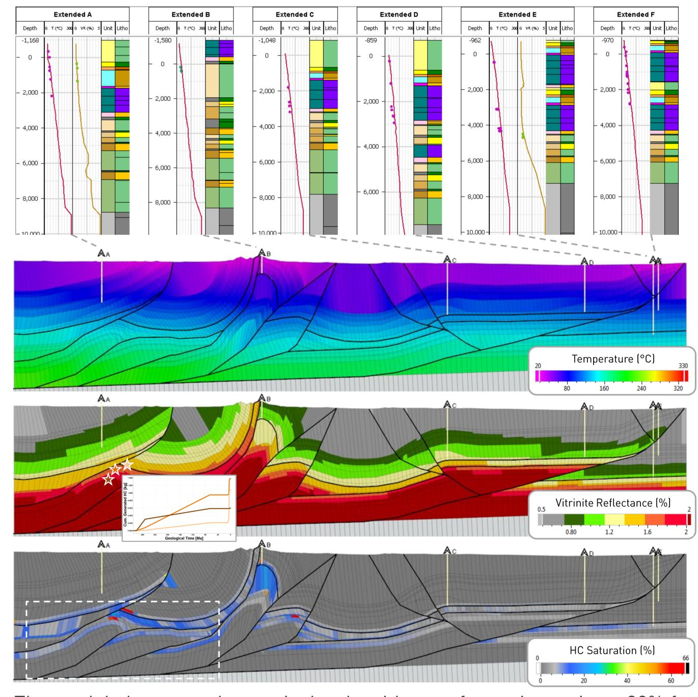
The model shows good maturity levels with transformation ratios > 80% for deepest source rocks. HC generation starts in Permian and is boosted in Pliocene with very high sedimentation rates. It leads to a favorable timing for HC trapping with deformation in the Western area where we observe accumulations in structural and fault traps.
