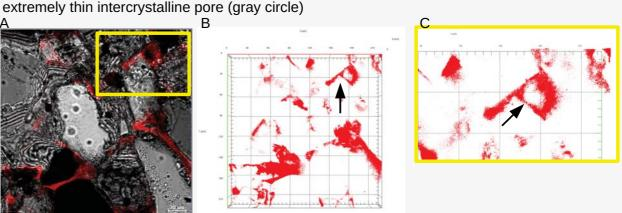
Interparticle porosity in this image (center of yellow box in A) is connected to the intercrystalline pore network (arrow in B), providing additional storage and connectivity (arrows in B and C)
