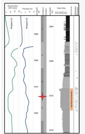
The Williston Basin sample is from the Middle Bakken Formation. The dolomitic quartz arenite is the coarsest grained reservoir unit in the core. Grain size is commonly silt size to vf sand size. Dolomite is common as a cement and replacement mineral, occluding most of the primary porosity visible using standard optical microscopy.
