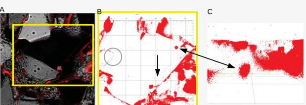
Dolomite rhomb in center of image exhibits minor intracrystalline porosity at margin (arrow in B). Note the isolated several-micron-scale pore (double-headed arrow in B, C). The pore throats giving it connectivity are likely beyond resolution of confocal method. Also note the
