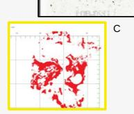
Intercrystalline pores (red) outline the euhedral crystal boundary (middle arrow in A). Interparticle pores (top, bottom arrows in A) are present. A rare region of intracrystalline pores present (C)
