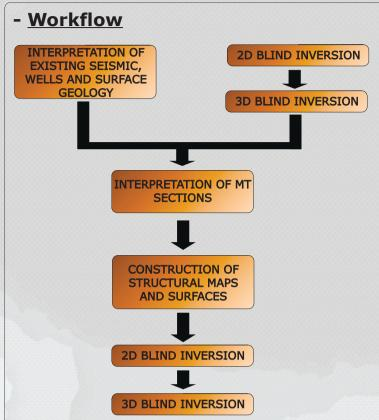
The interpretation process began with the generation of a geological model based on the 2D seismic information, the geological map, dip and azimuth data from the surface, and the well data. Secondly, the MT - Resistivity sections were added to the interpreted sections in order to compare both responses. Then, the geo-electric sections and seismic sections were correlated. Finally, once the information was confirmed it was used as the input for the constrained inversión.
