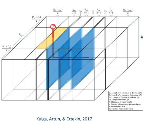
Discrete fracture network (DFM) modelling is the most widely applied approach to model shalegas reservoirs where the entire reservoir is discretely created, including the network fractures, hydraulic fracture, matrix blocks, and unstimulated areas. However, DFM modelling increases computational time, creates potential convergence and stability issues, and building a grid design with local grid refinements is laborious and can be timeconsuming.
