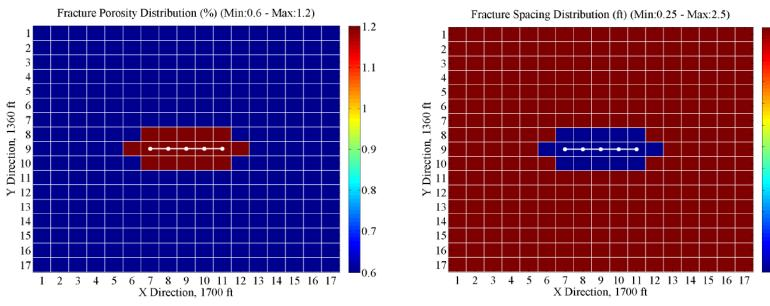
In this history match, reservoir area is kept relatively small as well as the horizontal wellbore length and hydraulic fracture dimensions to match the proposed initial flow rate, which is 1 MMSCFD. It is calculated that the daily production average error of field data versus PSU-SHALECOMP is 7.8% and the average error values for cumulative volume is 1.2%.
