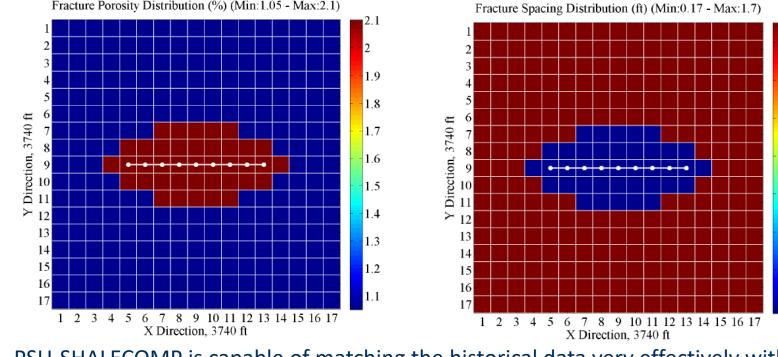
PSU-SHALECOMP is capable of matching the historical data very effectively with the combination of SRV approach. It is calculated that the daily production average error of field data versus PSU-SHALECOMP is 5.9% and the average error values for cumulative volume is 0.7%.
