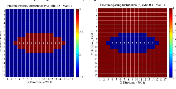
Again, PSU-SHALECOMPs results had a near-perfect match against the normalized field data using the SRV concept. This model is rather large in terms of area. It can be seen that the well will produce nearly 2 MMSCFD at the end of the 20th year, making it highly economical. It is calculated that the daily production average error of field data versus PSU-SHALECOMP is 7.2% and the average error values for cumulative volume is 1.1%.
