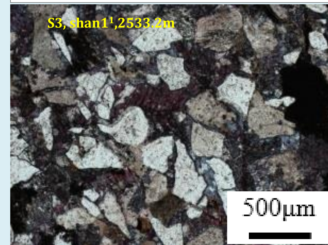
Lithofacies5: Tightly carbonate-cemented sandstone
