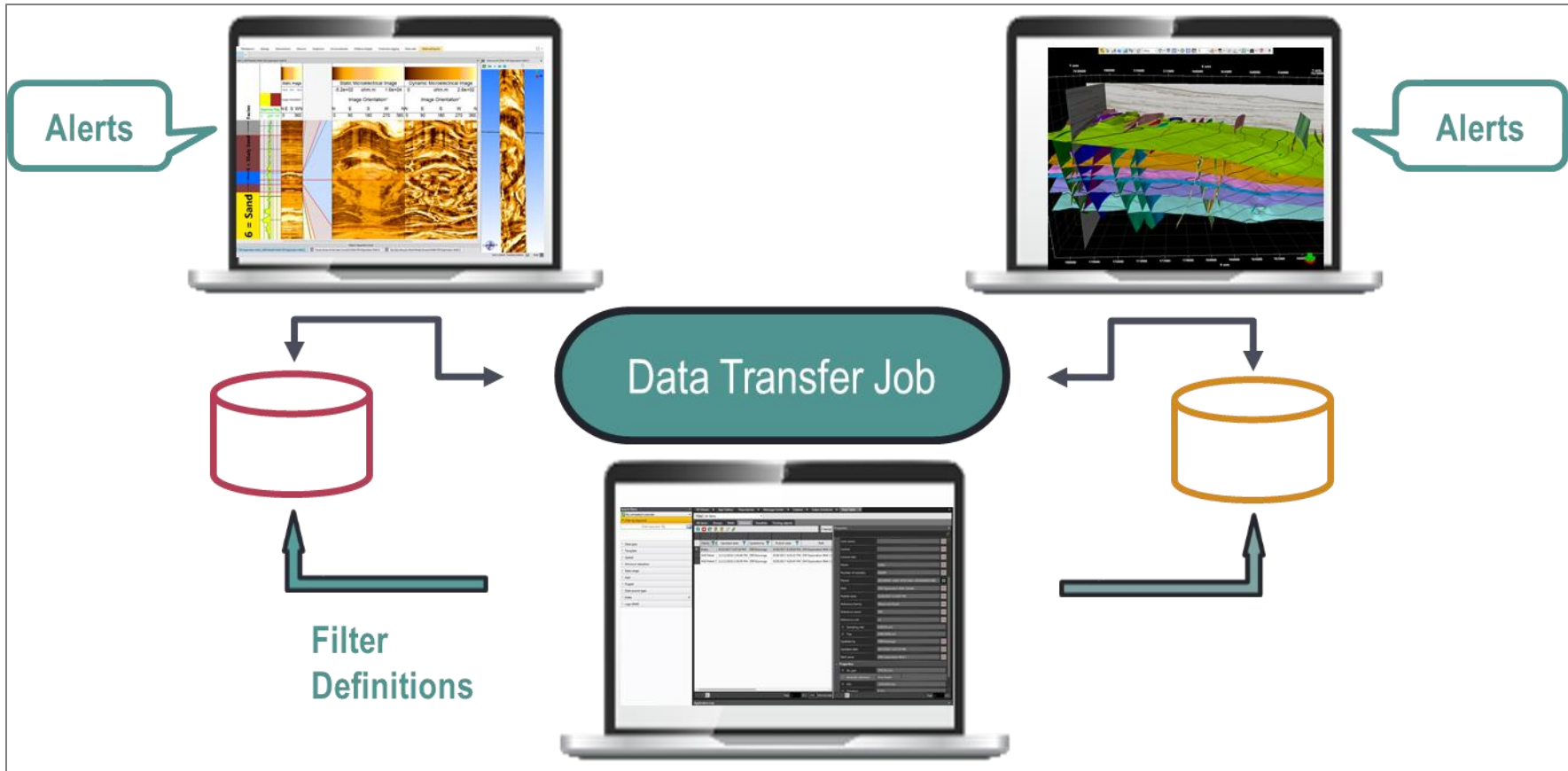
Figure 11. When a data item is updated in the shared-earth platform (left, red cylinder), it will be automatically copied to the shared-wellbore platform datastore (orange cylinder) by the job management system based on the job rules. After the item is in the target system (here the shared-wellbore platform), the end user can choose to be notified of the update based on filter rules configured by the collaboration system.
