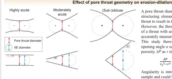
A pore throat diameter corresponds to the diameter of the structuring element (SE) when a pore breaks up at its throat to result in two smaller pores.
