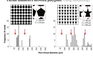
Pore throat diameters are inaccurately measured where different throat angles occur on the image. Higher angularity results in overestimated diameters.
