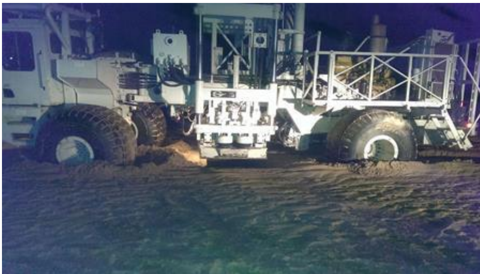
Figure 7. Vibrators stuck in Sabkhas.
