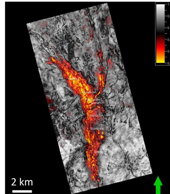
Sw minimum amplitude map overlaying variance map over Scarab channel 1 reservoir
