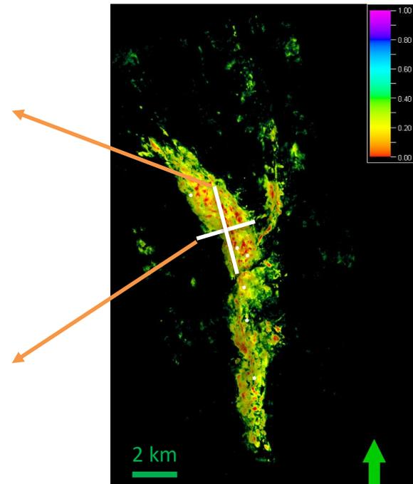
Sw min. amplitude map over Scarab channel 1 reservoir
