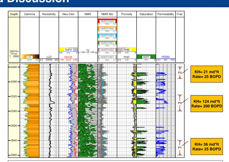
Well example: Connected KH through frac and rate observed against different intervals
