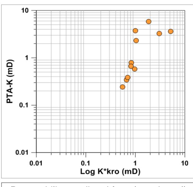
Permeability predicted from logs tie well with the same obtained from PTA analysis of well tests
