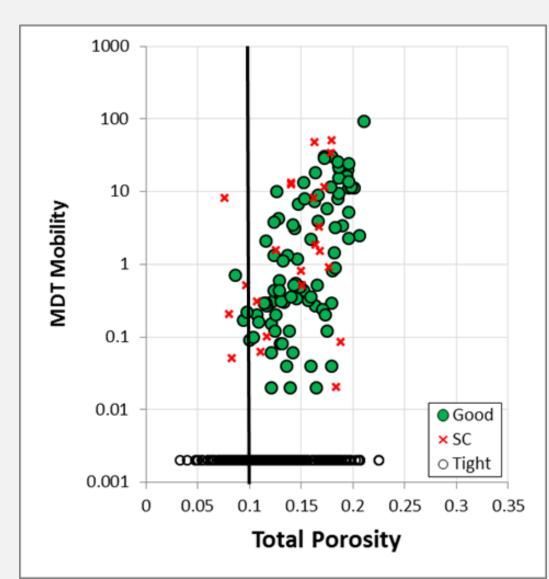
Reservoir cut-off used in V&V field: PHIT>=10% & VSHALE<=55%
