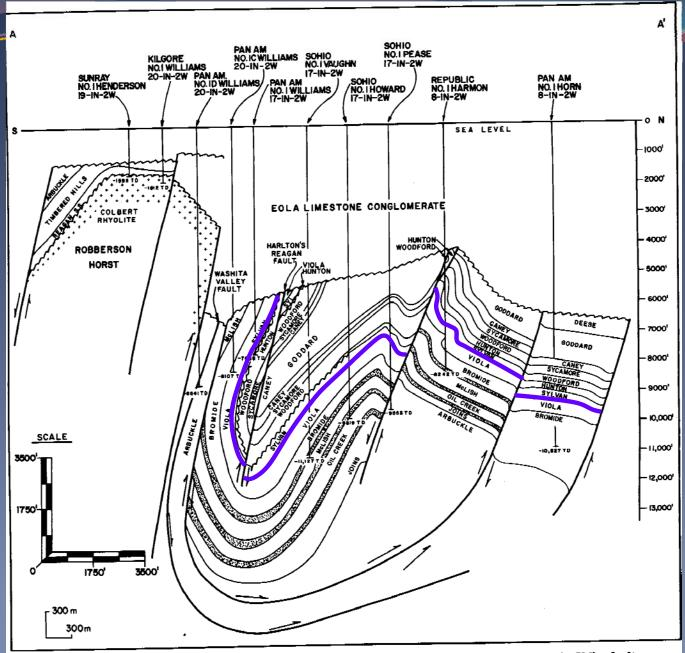
FIG. 6—Cross section AA', Eola field, from Harlton (1964); revised. Multiple fault types occur in Washita Valley fault zone.
