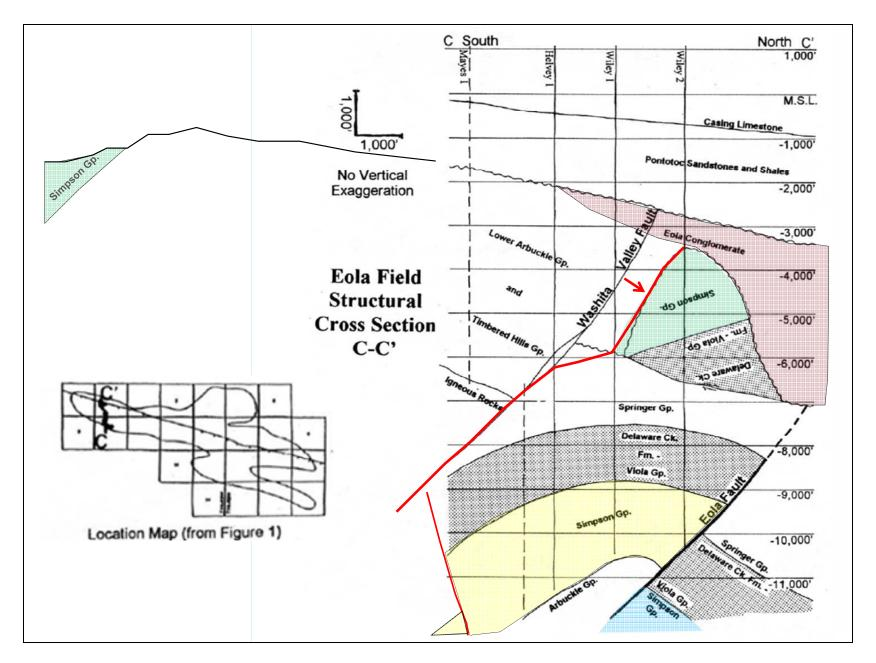
Presenter's notes: The Eola Klippe is a thrust sheet that came across much of the Eola structure north of the Eola Fault. It can be more than 3000ft thick and has well developed Bromide sands and Bird's-eye lime as well as Viola, although they are most commonly inverted. Whether present and trapping, these sands can produce in excess of 100,000 BO per well.
