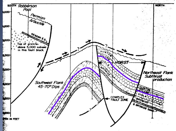
3—Eola has over 3,000 ft. of relief; on the northeast flank oil is trapped against a reverse that has between 800 and 1,400 ft. of throw.
