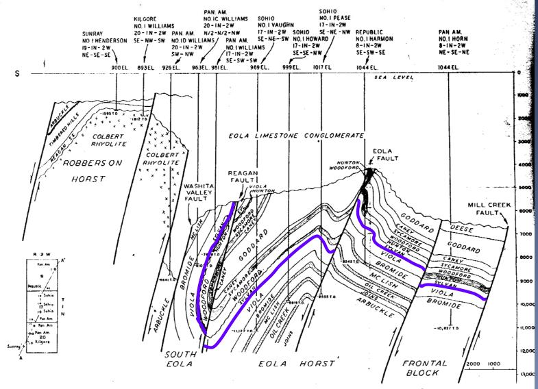
Fig. 6.--Structure sections, Eola field, Line A-A' from southwest to northeast, through secs. 19, 20, 17, and 8, T. 1 N., R. 2 W. (Fig. 5).
