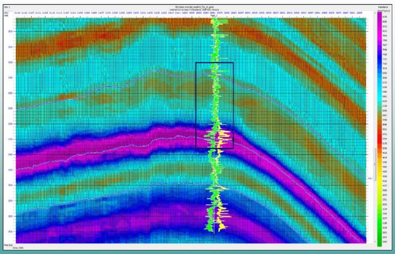
Vertical (inline) section with P-impedance as a result of seismic inversion. The color scale represents impedance values. In the middle of the section two logs are plotted along a well: in yellow P-impedance and in green total porosity.
