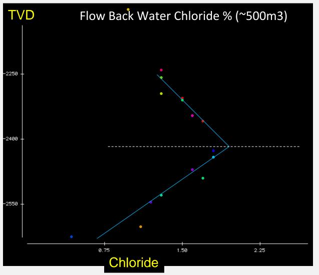
Normal increase of chloride content with depth as expected in a hybrid shale system
