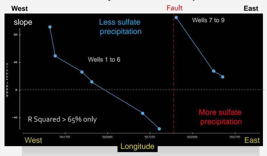
A plot of the Ba-Cl slopes against longitude (X) clearly demonstrates the near West-East distribution of the Ba-Cl trends in the Upper-Upper Montney.
