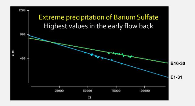
Slopes calculated per well using all flowback water analyses. The diagram displays a range of observed slopes for wells with **linear Ba-Cl trends** through time (**R squared > 65% used as a cut-off**).
