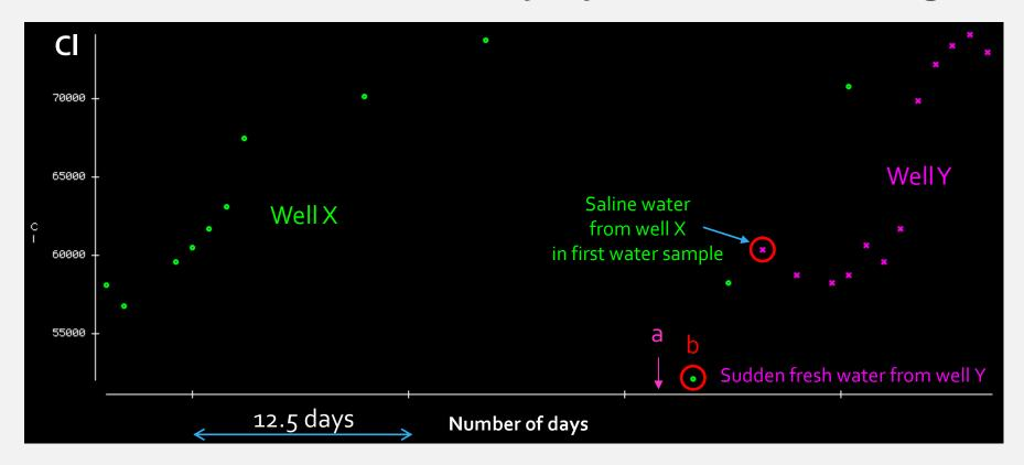
Well Y has interfered with the water flowback from well X: salinity went back to near frac water salinity and started an increase cycle from that point onward.
