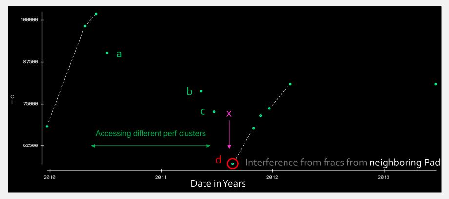
Very low salinity and start of a new salinity increase cycle in an Altares well is interpreted as linked to water breakthrough from Wells from another pad which have respective final completion dates of August 18 and 19<sup>th</sup> 2011 ("x" on graph)
