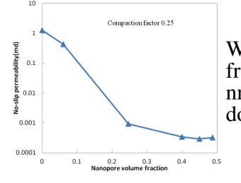
When nanopore volume fraction reaches 0.4, nm-scale pore networks dominate the flow path.
