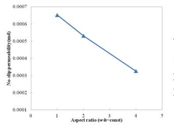
When all nanopores are sheetlike, higher aspect ratio reduces shale no-slip permeability.
