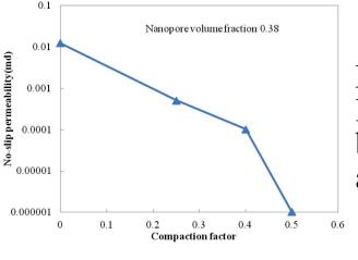
Large compaction factor leads to low connectivity between OM particles and clay agglomerates.
