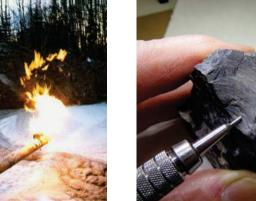
Gas flare at a coalhed methane test well near Houston, probably the Houston 1 well or the Houston 3 well. This photo was obtained in 2000 or thereabouts from the Lapp Resources, Inc. web site. The company and the web site no longer exist.
