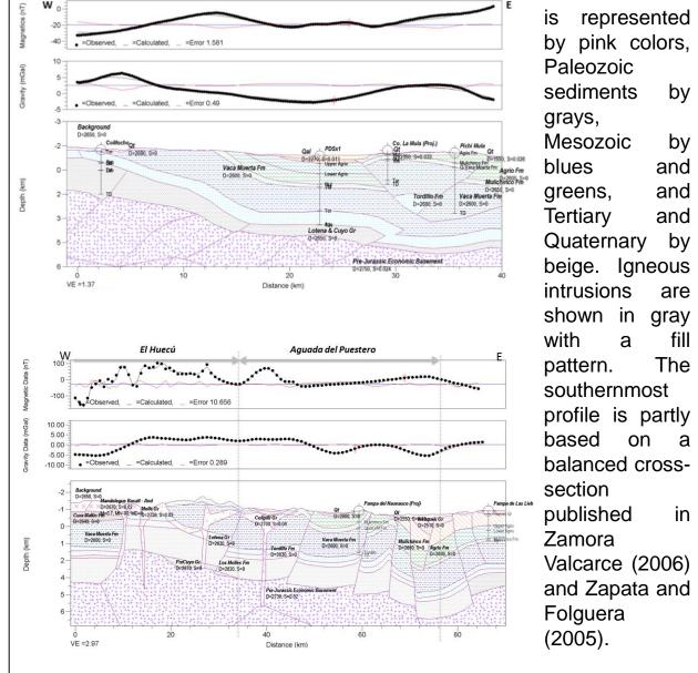
The black circles in the panels above the section represent the input magnetic and gravity data profiles, respectively. The black lines in the top two panels represent the values calculated from the models; the red line represents the error between the two. This caption is applicable to all profiles.
