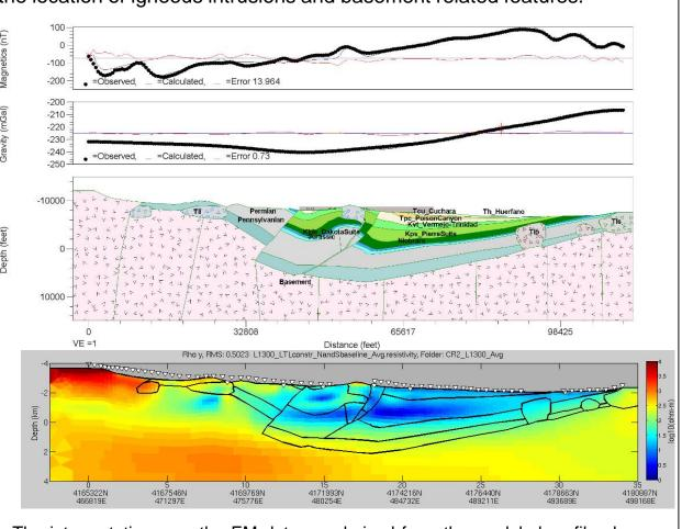
The interpretation over the EM data are derived from the modeled profile above. Note the agreement in low resistivity areas (blue) and sedimentary basin and higher resistivity zones (red and yellow) in agreement with igneous intrusions and basement related features.
