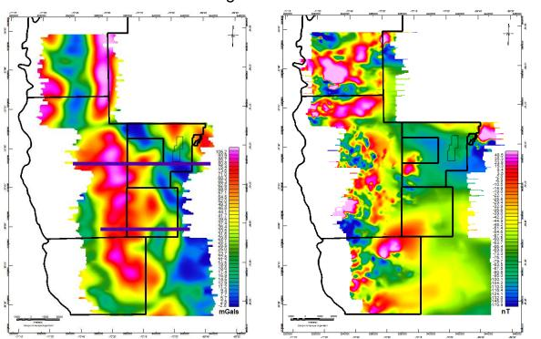
The positive anomalies observed in the gravity data reveal basement related features close to the surface. These are also observed in the magnetic data, where volcanic plugs and intrusions are evident in the western portion of the survey. All profiles were constrained by surface geology and, where available, well log information. The average density and susceptibility values used for each interval are shown in the profile.
