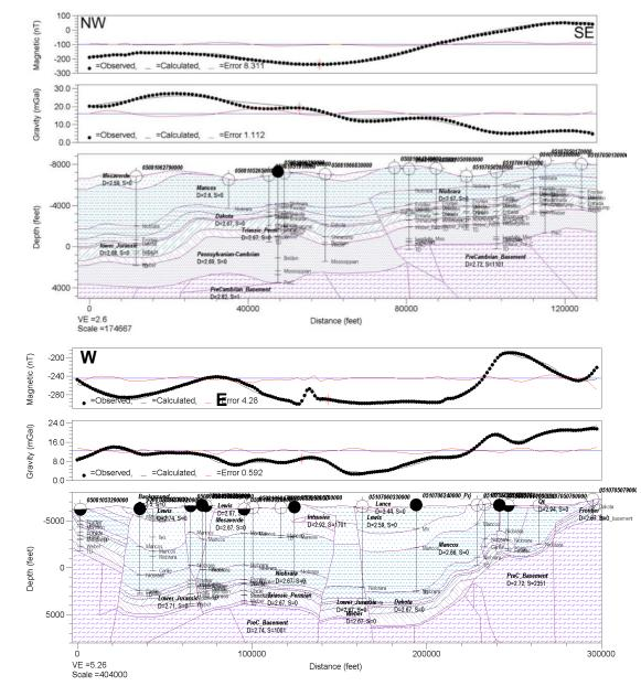
The magnetic and gravity data reveal, not only irregular topography of the basement, but also lithology contrast, as observed in outcrop.
