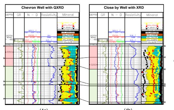
There are inconsistencies of XRD measurements and reporting from different companies. Use public data with caution when calibrating mineral model. Only QXRD data is used in this study, Figure 4a.
