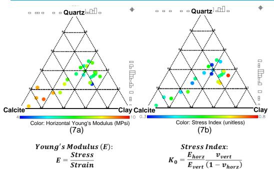
Comprehensive QXRD and triaxial tests from full diameter core have shown strong relationships between
