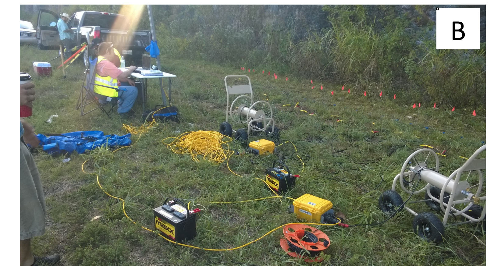
Figure 6: (A) Geonics Geode Seismograph paired with a computer for acquisition. (B) Photo of our seismic survey set up at the Pedro Survey area. The two yellow boxes are the connected seismographs hooked to battery power sources. In the background the flags mark where the single channel geophones have been placed. The MARkUP team member in the upper left is sitting at the table with our laptop for acquisition.
