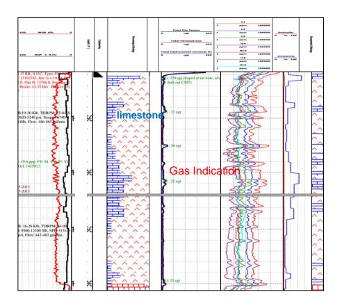
Figh Gamma-Ray readings correspond to limestone layers, and not shale as confirmed from mud logs
