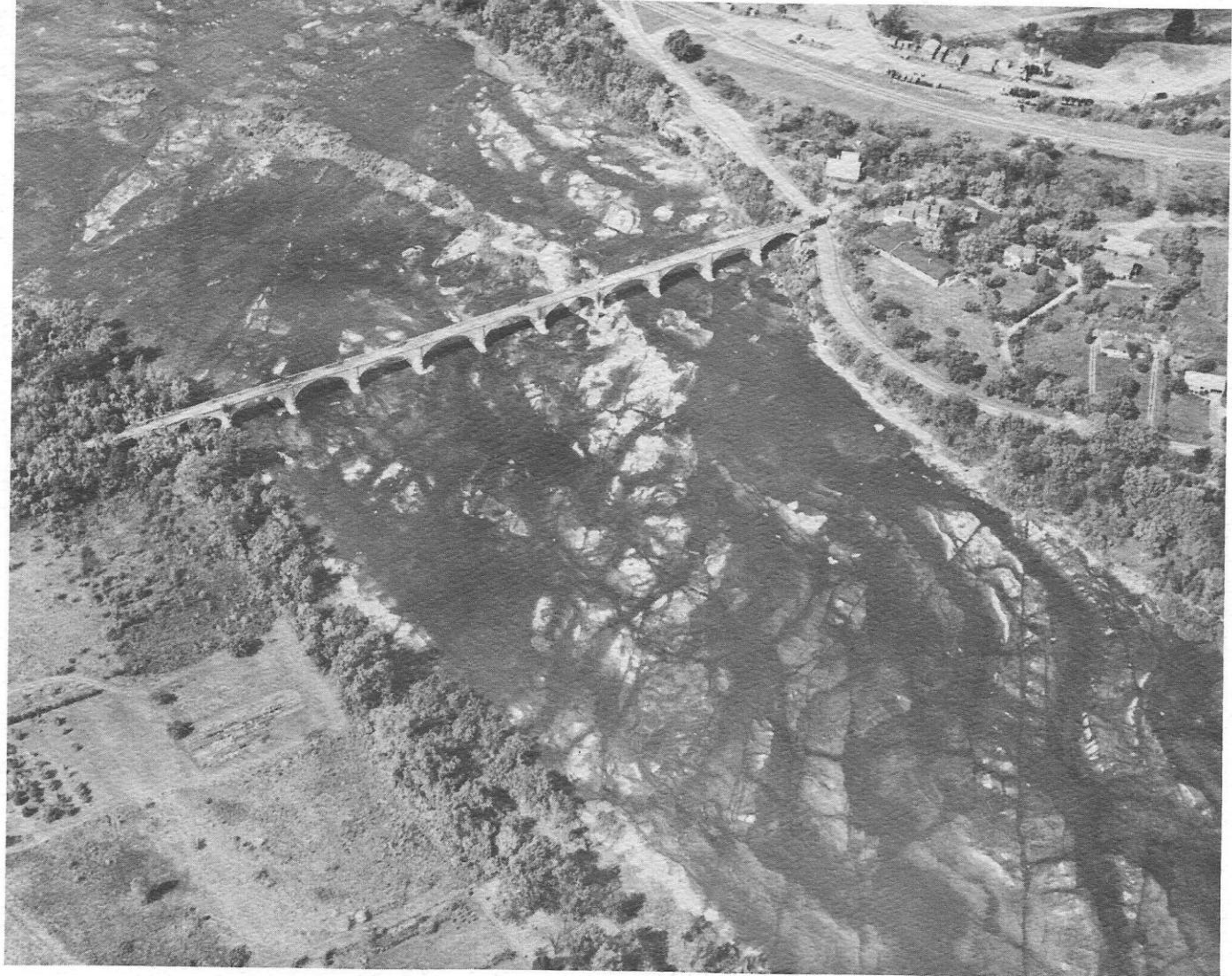
FIGURE 27.—Aerial photograph taken during drought of 1934 showing fault and fracture traces in the bed of the Maumee River along the Bowling Green Fault Zone. Southern edge of the France Stone Co. Waterville quarry is in upper right of photo. Forst Road bridge over the river is oriented N-S. Photo courtesy of the Ohio Historical Society.
