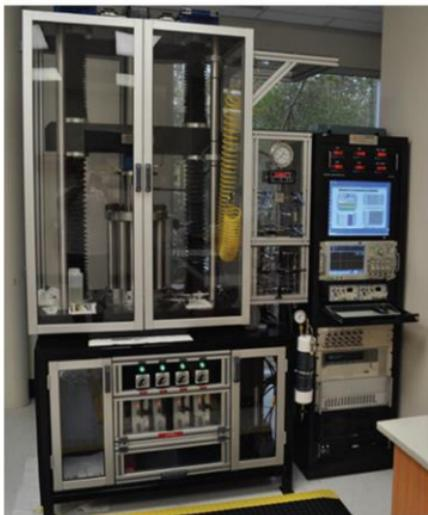
Triaxial testing of core for elastic properties and strength
