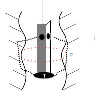
Wireline Tool collects sectored compressional data from within the borehole in time (we, in our processing, correlate time with depth). It is assumed that the standard depth of investigation is 6 inches.
