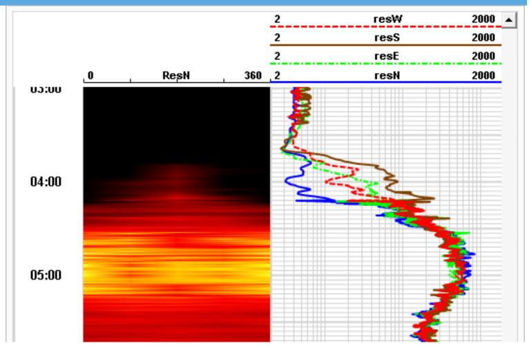
This example from Mississippi Lime shows how resistivity imaging and dip calculations are possible from the four basic measurements.
