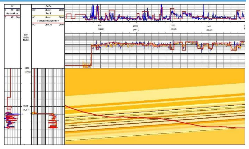
Thin sand-shale sequences 20 - 200 ohm.m. have nano-Darcy permeability. LogXD software computes bed-boundaries & layers using forward tool model
