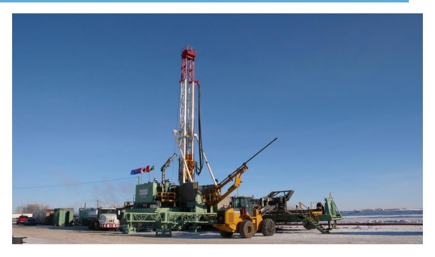
Shallow (420 m.) laterals are drilled with a Super-Single rig and completed in a few days.
