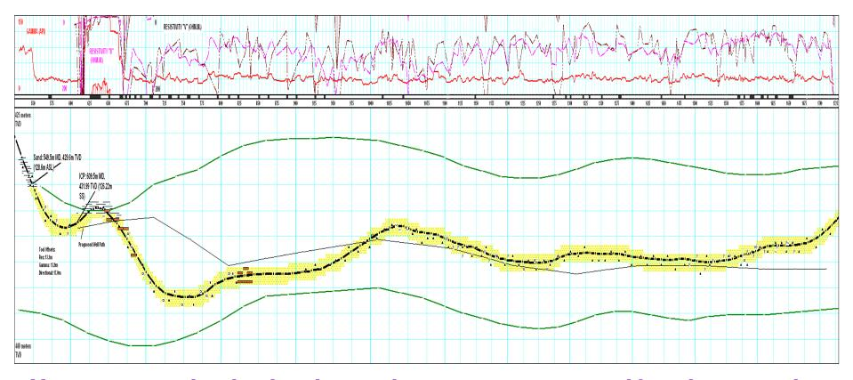
Upper sand-shale boundary unexpectedly located close above the landing point, causing slight excursion into water-wet shale, but most of the borehole is in the sweet-spot and productive.
