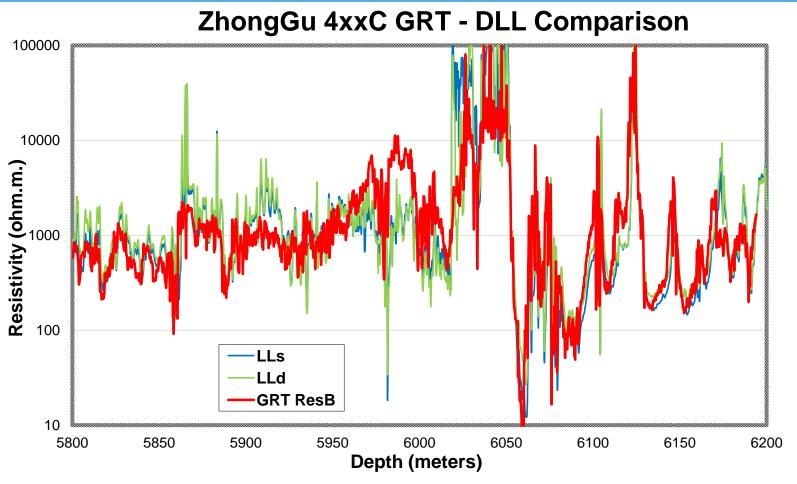
High-resistivity target is 100 - 20,000 ohm. meters Memory log from GRT shows good correlation with wireline Dual-Laterolog, and could replace it.
