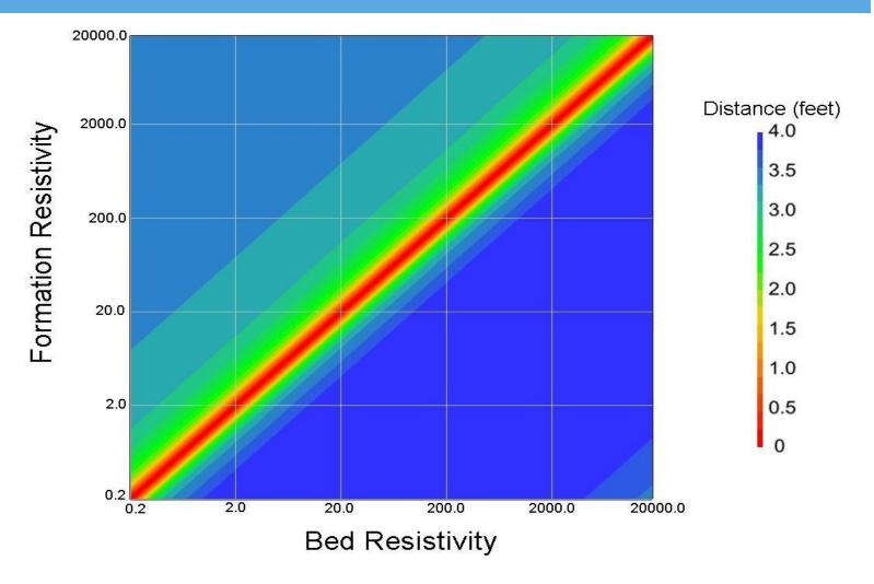
Maximum bed-boundary detection distance is about one meter from the borehole for contrast > 3:1
