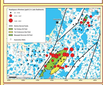
Distribution of headspace nPentane (C5) in lake sediment samples over and around the Tuk and Mayogiak oil and gas fields. There is good spatial correlation of the nPentane anomalies with the Tuk and Mayogiak oil & gas fields. Anomaly contrast is about 2.
