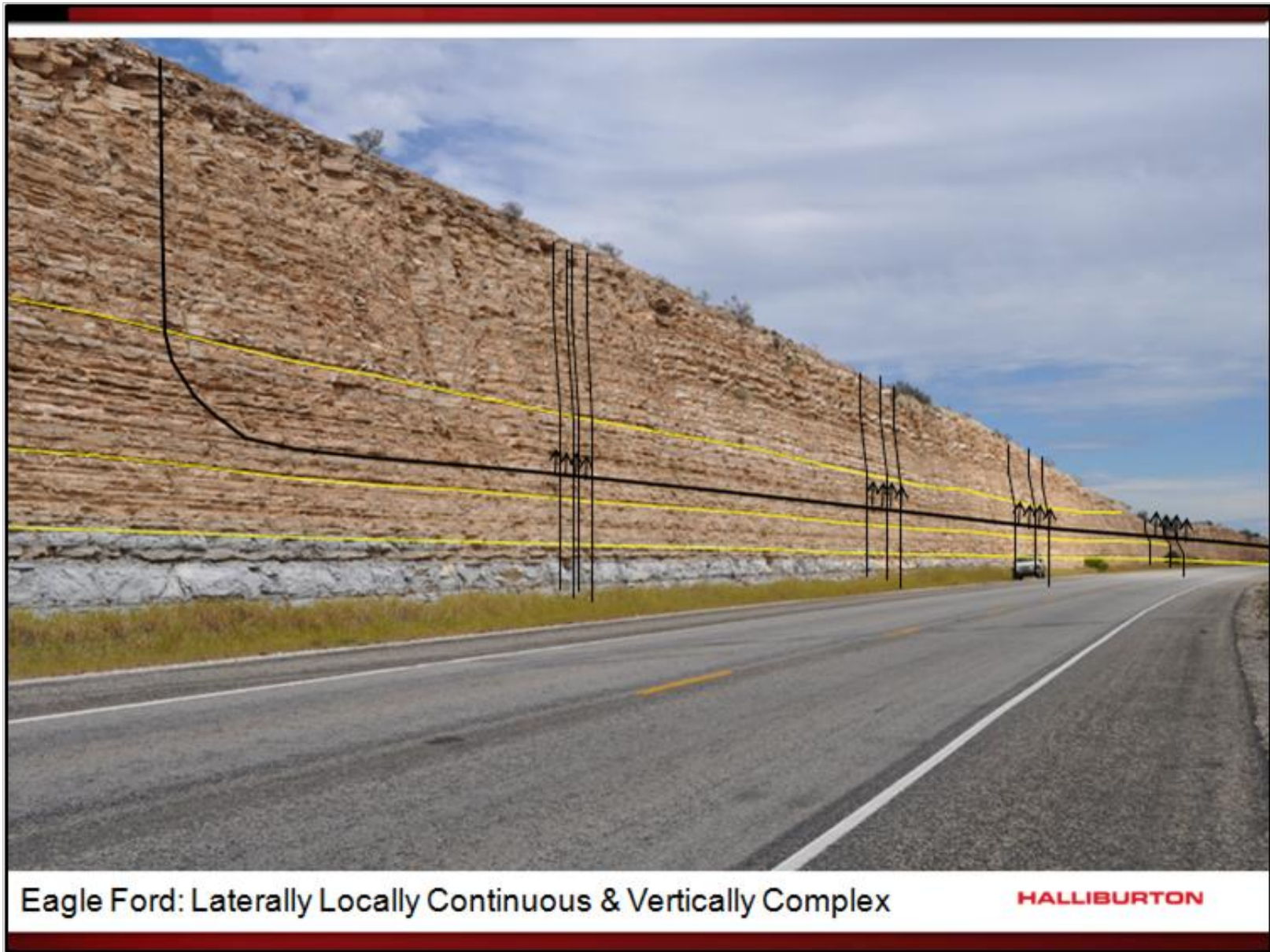
Figure 1. Eagle Ford outcrop and superimposed horizontal well with fracture treatment stages.
