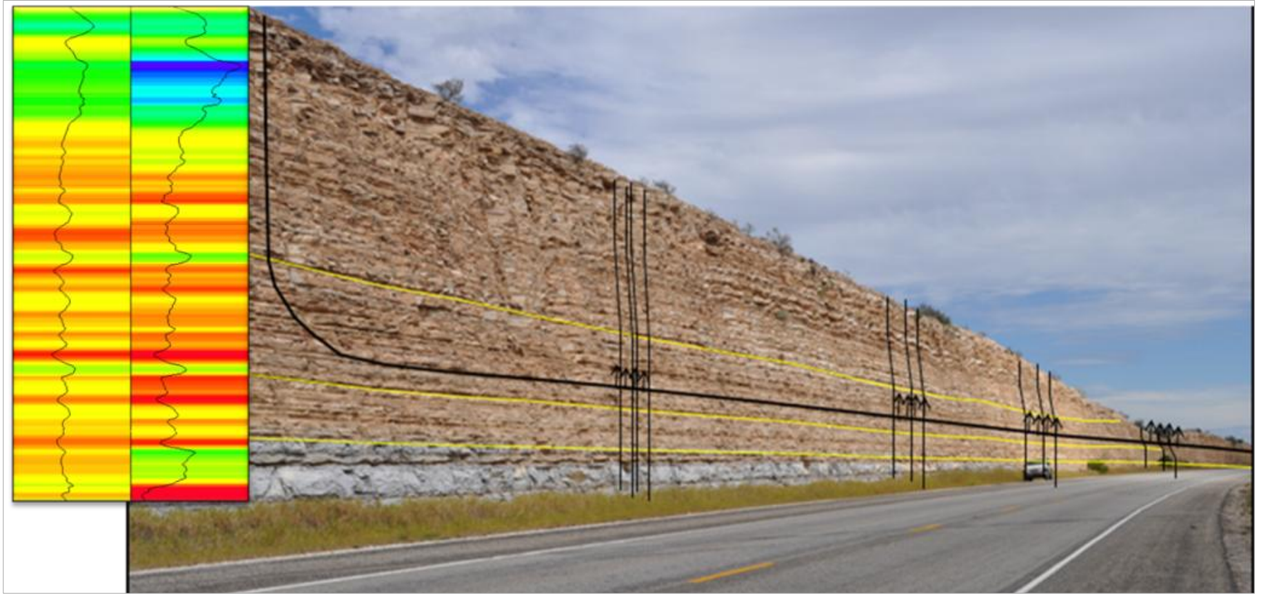
Figure 5. Eagle Ford outcrop with dipole sonic solution of vertical and horizontal closure stress.
