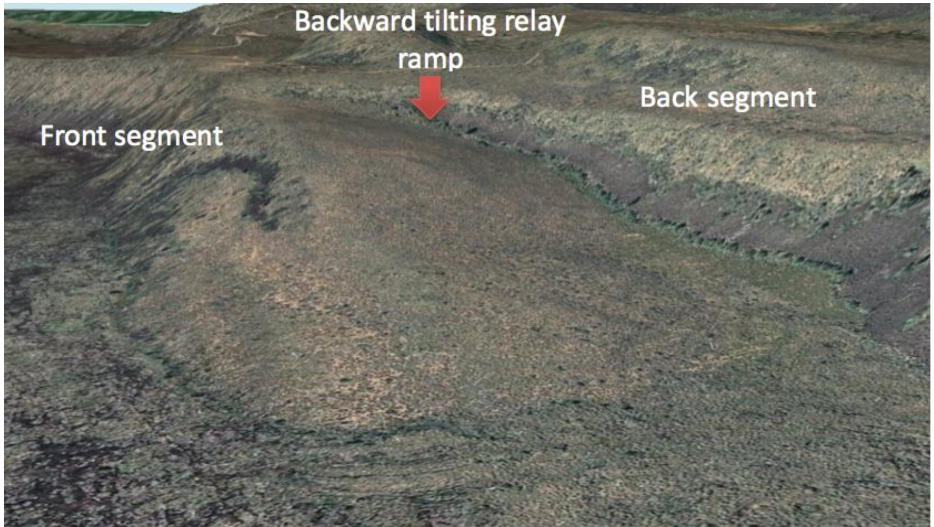
Figure 1. Google Earth image of a backward tilting relay ramp along the Hat Creek fault, California. The change in elevation of the ramp from the front segment to the back segment should be subtracted from the combined throw from each segment to obtain the correct cumulative throw across the fault near the relay ramp.
