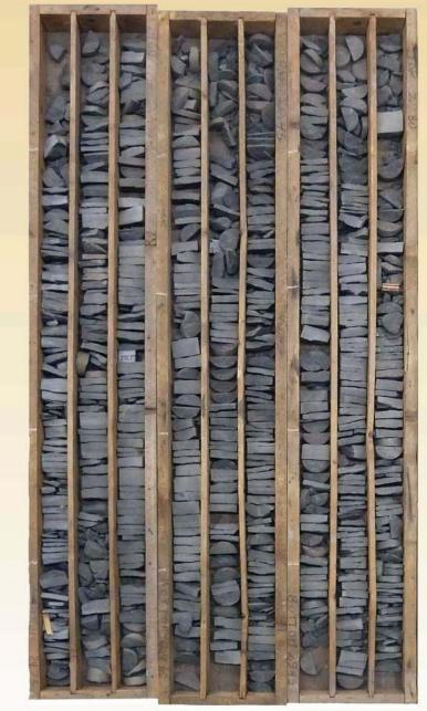
Typical Macasty shale in Princeton Lake drill core showing massive, dark-coloured, fined-grained ithology with poorly developed fissility. Core shown here in 5-feet segments.
