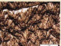
Photomicrograph showing cone-in-cone horizontal structure within the Macasty mudstone with concentric cones nested inside each other and thin layers of clay trapped between cones. These features formed by expansive mineral growth of cone-shaped aggregates of fibrous calcite. Scale bar is 1 mm.
