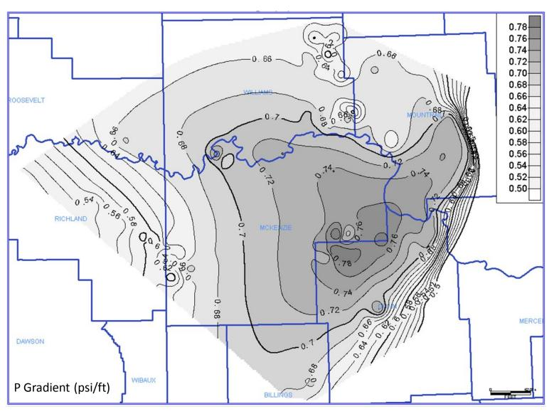
**92 BHP and DFIT data points** + 6 hydrostatic points at eastern margin + 6 Sanish-Parshall points
