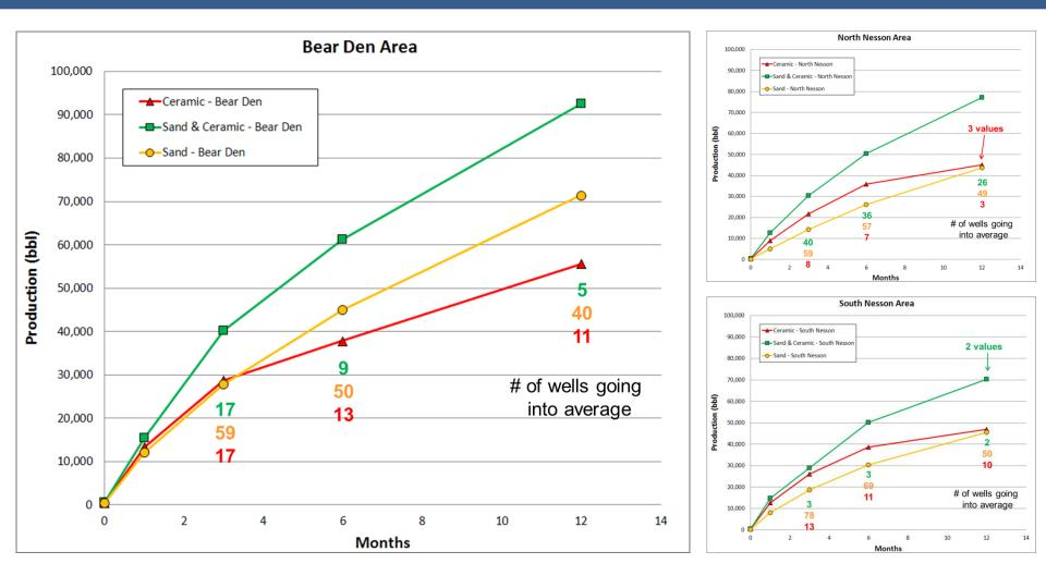
Despite ceramic being a superior proppant, a mixture of about **2/3 sand and 1/3 ceramic** proppants yielded better production results than either sand or ceramic alone (based on this limited dataset)
