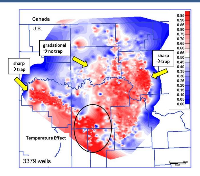
Oil / (Oil + Water) ratio based on cumulative production
