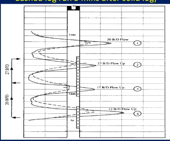
(Well on injection into perfs; tracer at point 1; 5 logs run 30 mins apart; flow behind casing into Sand C)
