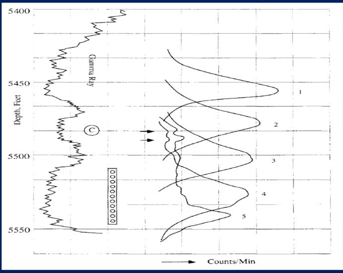
(Well on injection into perfs; 5 logs runs presented on separate logs; flow behind casing into Sand C)
