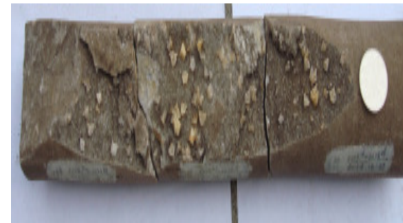
Semi-filled vertical fractures, 2278.94~2279.29m, Xu 2 Member, Hc 5 Well
