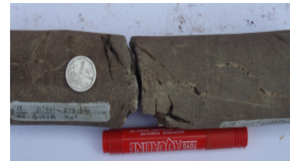
Semi-filled vertical fractures, 2179.03~2179.26m, Xu 2 Member, Hc 7 Well
