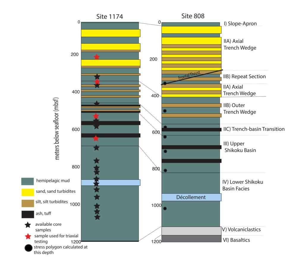
Site 1174 and Site 808 are located along the Muroto Transect in the Nankai Trough, offshore SW Japan. Site 1174 and Site 808 are within 2 km of each other and are thus very similar stratigraphically. Structurally, Site 808 is in the frontal thrust, whereas 1174 is in the protothrust. Site 808 has a repeat section where it crosses the frontal thrust.
