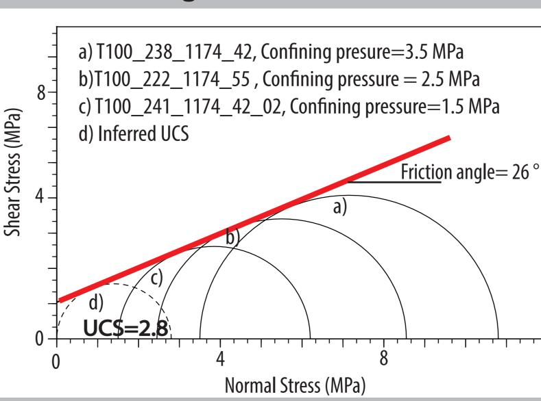
Axial stress at failure used to define failure threshold. UCS determined form fourth circle at 0 confining pressure.
