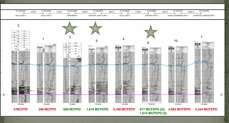
Initial four wells on left landed lower in Marcellus section: all low IP's. Four laterals on the right landed higher in section with major changes in results. Landing point/target = Major driver!
