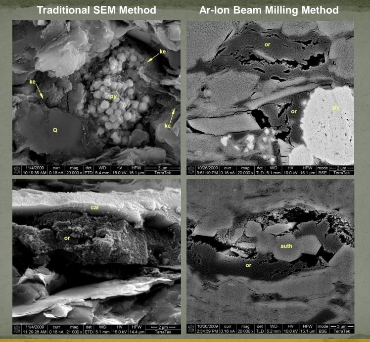
Use of Ar-Ion Beam milling techniques greatly aiding in showing role of organic porosity over standard 2D SEM
