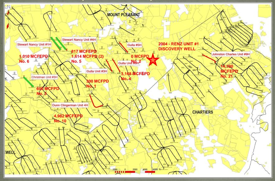
First three lateral wells tested 0 MCFPD to 600 MCFPD. Fourth and afterwards tested 1614 MCFEPD to 14,100 MCFEPD...What was the driver? All have similar azimuths and length. Initial laterals in liquids rich portion of play highlighted in green and were among the first laterals in the play.
