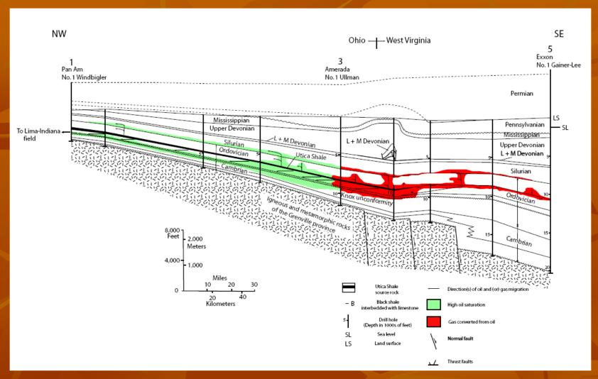
Gas-prone areas of Utica Shale will be in the deeper portion of the basin. Much of Ohio may contain appreciable amounts of oil and natural gas liquids within Utica wells as illustrated by this NW–SE-oriented schematic cross section by Bob Ryder illustrating the results of geochemical analyses of well samples.
