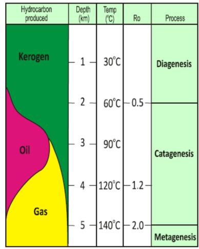
Figure 8. Graph of subsurface processes, depths, temperatures, and vitrinite reflectance values associated with the conversion of organic matter to hydrocarbons in petroleum source rocks. Modified from Tissot and Welte (1984).
