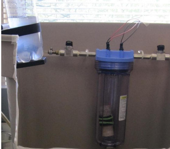
NaCl brine based on SCA guidelines. Core is evacuated and then saturated.
