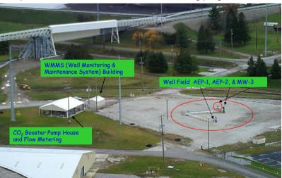
Approximately 37,000 tonnes CO<sub>2</sub> injected, with majority of injection in the Copper Ridge zone, which showed very good injectivity
