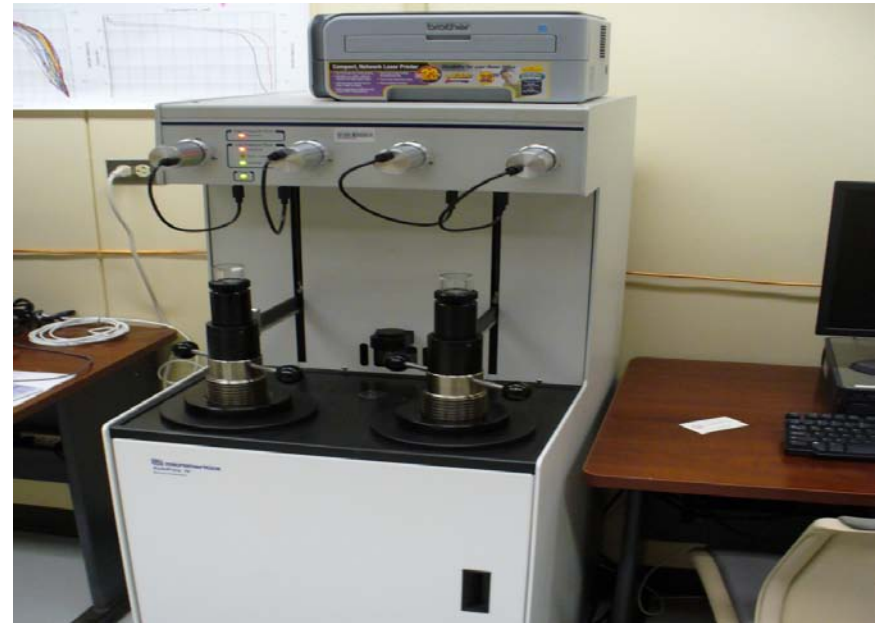
Mercury Injection Capillary Pressure (60,000 psi)
