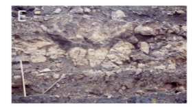
E. Outcrop of the Upper Pittsburgh Limestone exhibiting a nodular exposure interbedded with shale (Stewart Quadrangle). Meter stick at left for scale.
