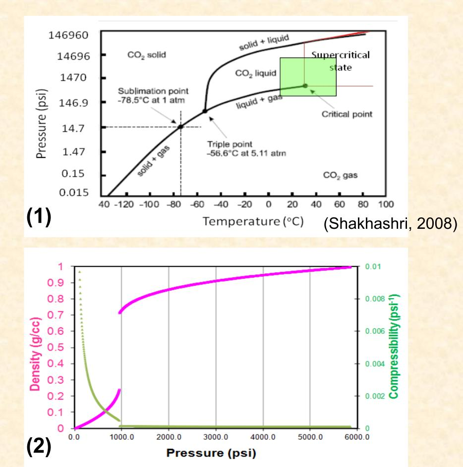
At reservoir conditions (Figure 1), expected CO<sub>2</sub> phase is shown by green region. Figure 2 is plot of estimated density and compressibility using Peng Robinson EOS.
