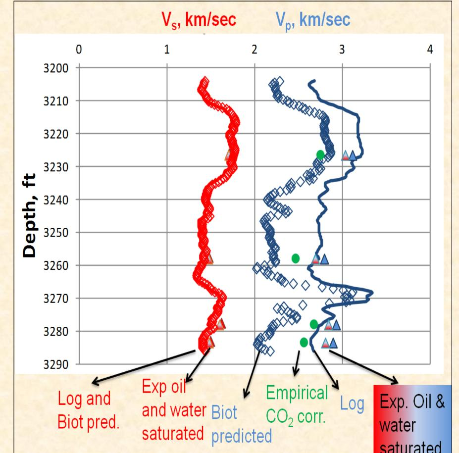
Pre-flooded log from a well 159-2 on the study field is plotted with empirical and Biot predicted elastic velocity values.
