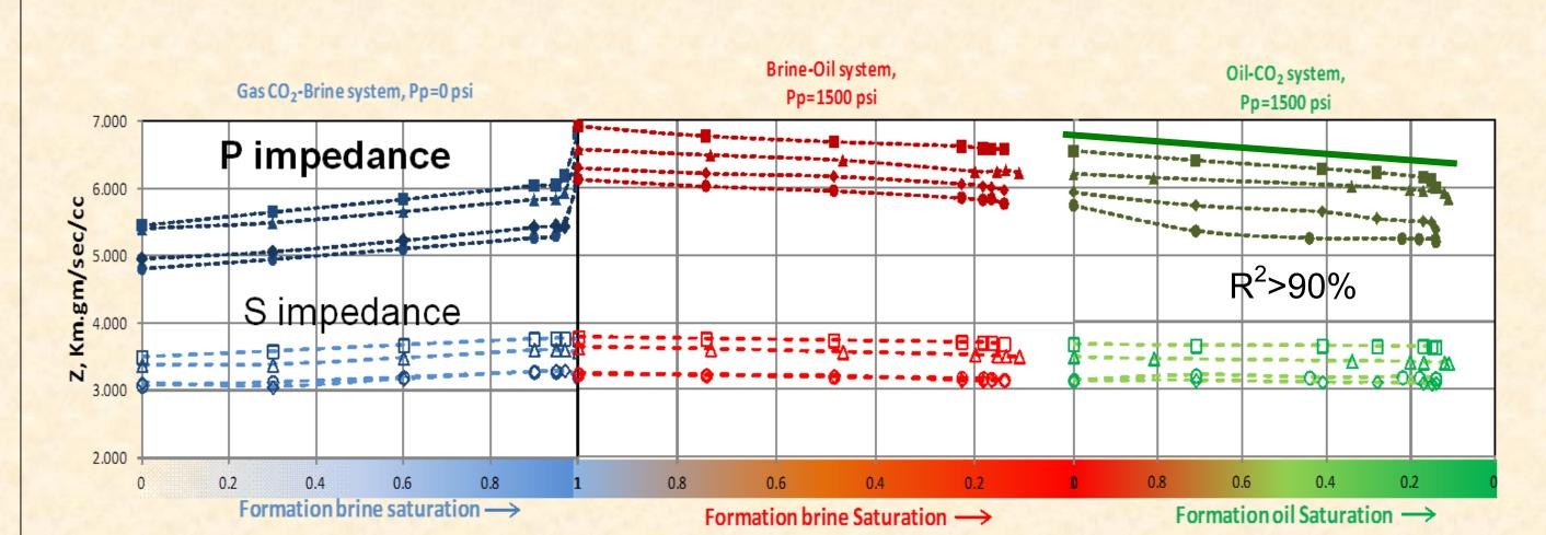
Linear regression analysis is performed on the experimental impedance data points in CO2 flooding scenario to generate an empirical relationship.
