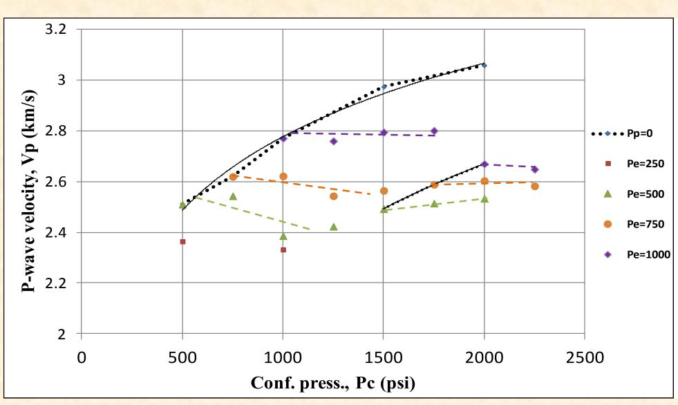
Elastic Velocities (P and S wave) are measured as a function of confining pressure and zero pore pressure. The pore pressure was incremented by 250 psi and variation of velocities with confining pressure were recorded, till pore and confining pressure of 1500 psi and 2250 psi respectively.
