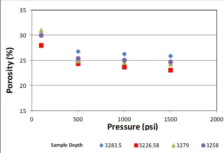
Drop of 18% (average) in porosity was observed with effective pressure when brought to reservoir conditions. This is one of the reasons why we perform the experiments at reservoir conditions.
