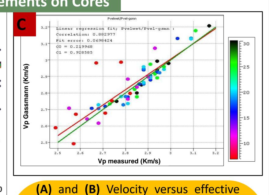
stress response of core data of core plugs from two wells. Dots indicate core measurements for brine saturated plugs. Solid curves judge against core and predicted response using Gassmann equation. (C) Vp predicted versus Vp measured cross plot as validation QC for Gassmann fluid substitution. Green curve is the line for perfect prediction. A red curve is the linear regression indicating 88% correlation between measured and predicted velocities.
