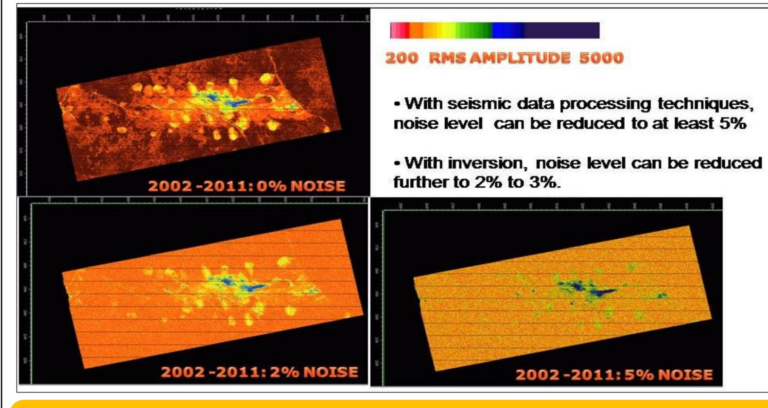
Random noise analysis was analyzed at the reservoir level with dominant frequency of 35hz. 0%, 2%, 5% and 10% random noise were modelled and synthetics produced. With 5% random noise 4D anomalies are detectable.
