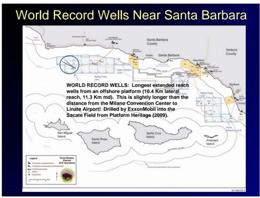
Presenter's notes: Highlighted here are some state-of-the-art technology in use on the West Coast. Although there are a few longer extended reach wells in the world, notably at Wytch Farm in England and off Sakhalin Island in Russia, they are from a land base and drilled into the offshore and therefore somewhat easier to drill.
