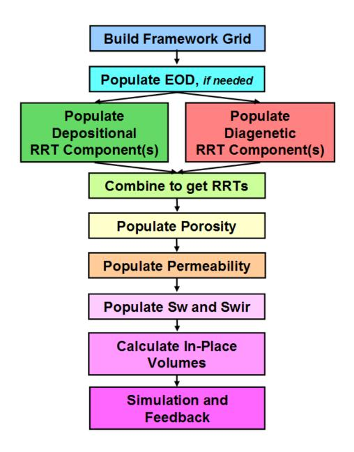
Figure 1. Preferred carbonate modeling workflow.
