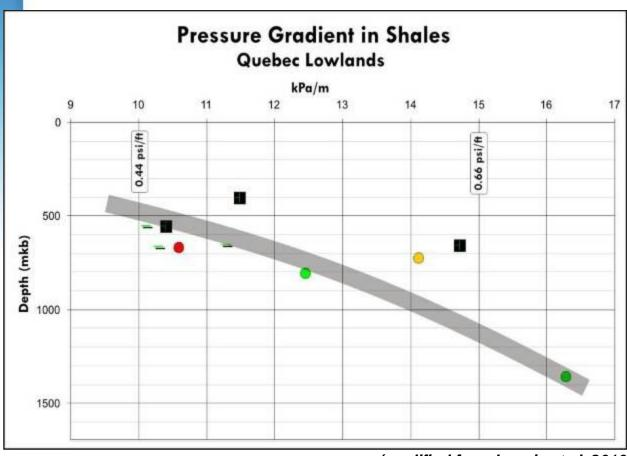
Pressure gradient data for some Shale zones over the Lower Décollement
